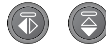
Left: mirror side to side button. Right: mirror end to end button.
